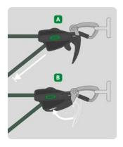
5. Pull excess line through tensioner [A] and close release handle [B].
